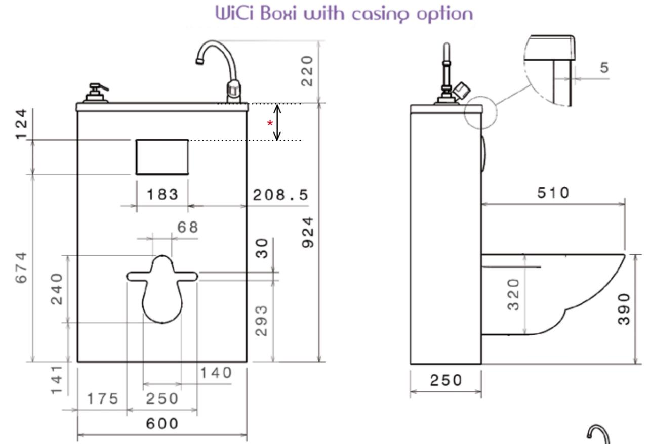
\*Required distance between the top surface of the Boxi support and the top surface of the basin: 11cm
